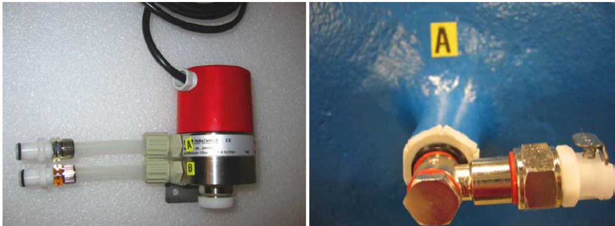
Figure 5.2. The differential pressure switch (left) and one of the connections on the filter body (right)
