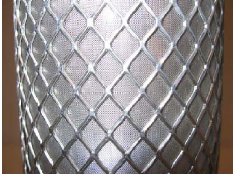
Figure 2.2. An expanded metal basket with a filtration degree of 0.1 mm
