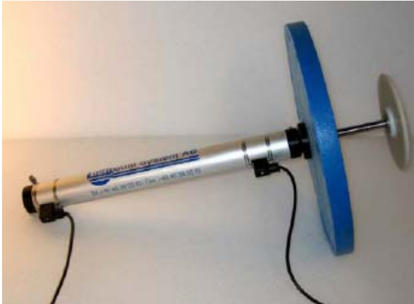
Figure 3.1. A cylinder with its disc for one of our smaller filters. At the ends of the black cords you can see the limit switches.
